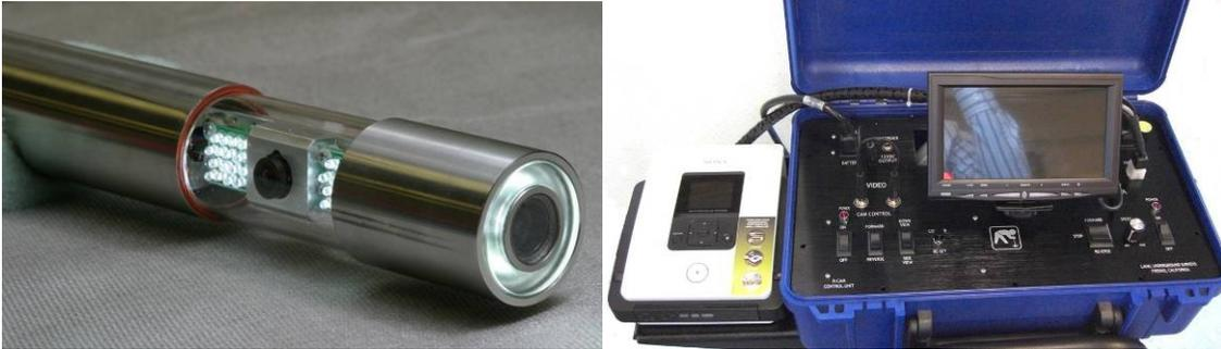
The R-Cam 1000 Color Video Water Well Inspection System is equipped with two cameras in a single housing, each with a wide-angle lens, for viewing down hole and side view images in water wells or boreholes. Low light level CCD sensors allow the cameras to detect images with minimal lighting power, as low as 1 LUX.
