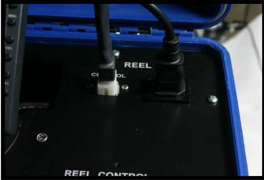
Plug the other end of the control cable into the control panel.
