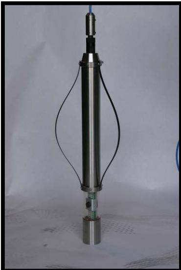
Thread the cable head through the centralizer and the cable head cover sleeve and connect the camera.
