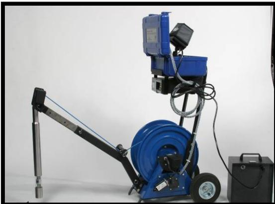
Connect the camera, battery and control cables. Do not power on until all cables are connected. Power off before disconnecting.
