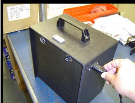
Plug the control cable into the reel.
