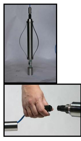
Thread the cable head through the centralizer and the cable head cover sleeve and connect the camera.
